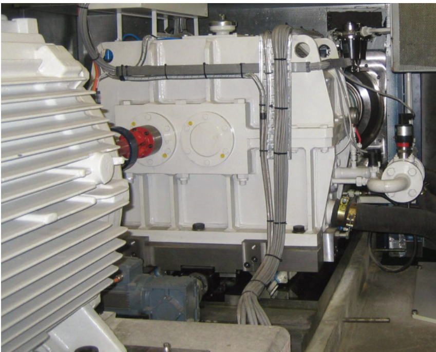
Drive system with motor, gear box, intermediate shaft and moving device
