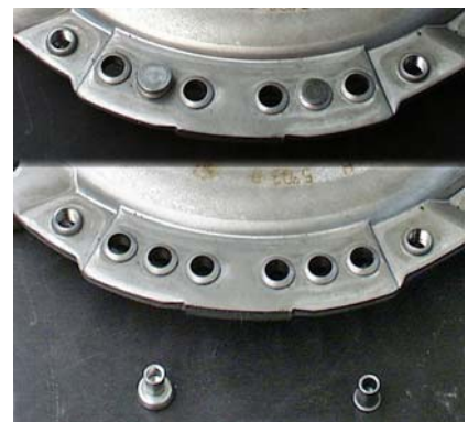
Rivets with different weights, inserted and calked at the top
