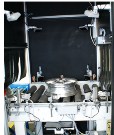
Inlet-conveyor with design detection
